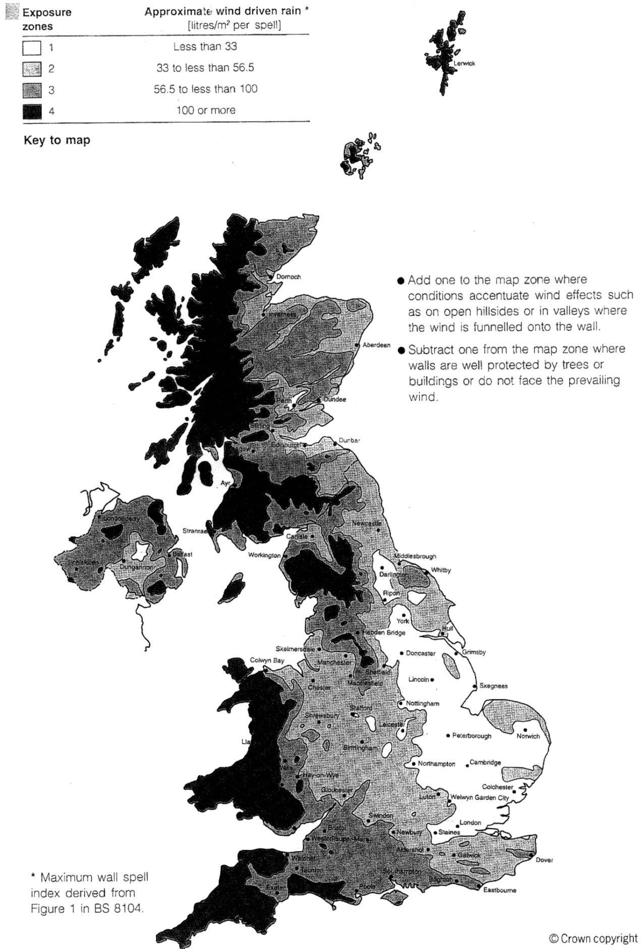
Fig. 28. Current wind-driven rain map (Graves & Phillipson, 2000)
